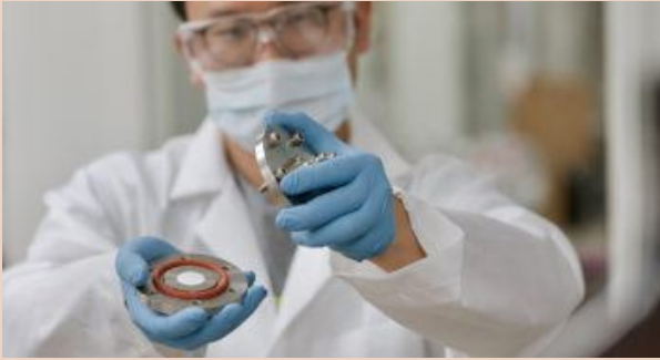
Dehumidifiers with enhanced polyimide membranes (white disc) will be energy efficient and have a smaller carbon footprint
