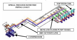
1. Eliminate long wet return line by installing the pump package just next to and underneath the Spiral Freezer. Only the long dry suction vapor come instead connecting pump package with the compressors. This will give the following benefit :
