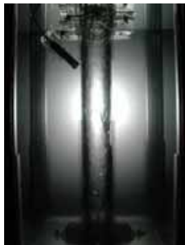
Figure 6(d) Example picture of annular flow
