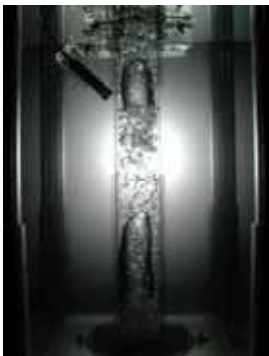
Figure 6(c) Example picture of slug bubbly flow, Re of U_L = 8000 , U_G = 100 mm/s
