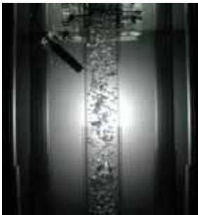
Figure 6(a) Example picture of core-peak bubbly flow Re of U_L = 8000 , U_G = 25 mm/s
