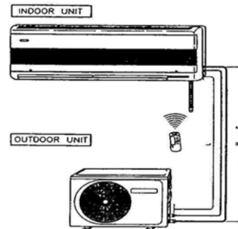
Fig. 2. Typical split system air conditioners (wall mounted)
